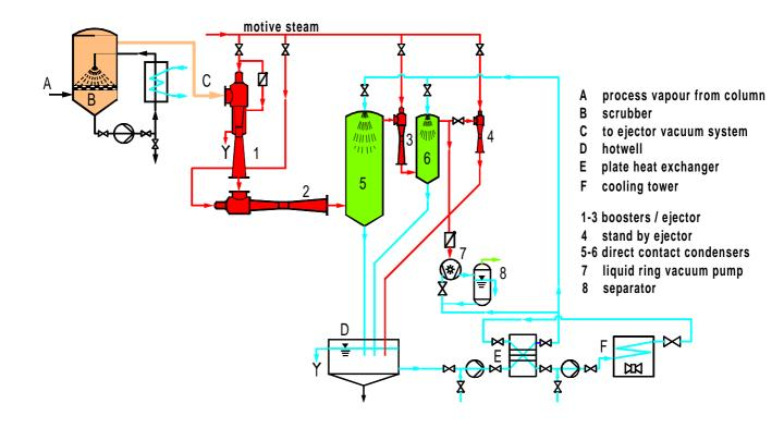
It is sensible in the case of multi-stage compressions to combine the advantages of steam ejectors and water ring pumps.
