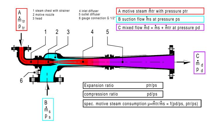
The compression attainable from the suction nozzle to the outlet nozzle is, dependent on the motive pressure, the specific motive steam consumption, and finally on the internal geometry of the ejector.
