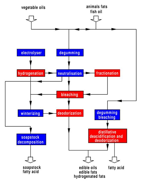
This picture shows the various process stages in the processing of edible oil.
