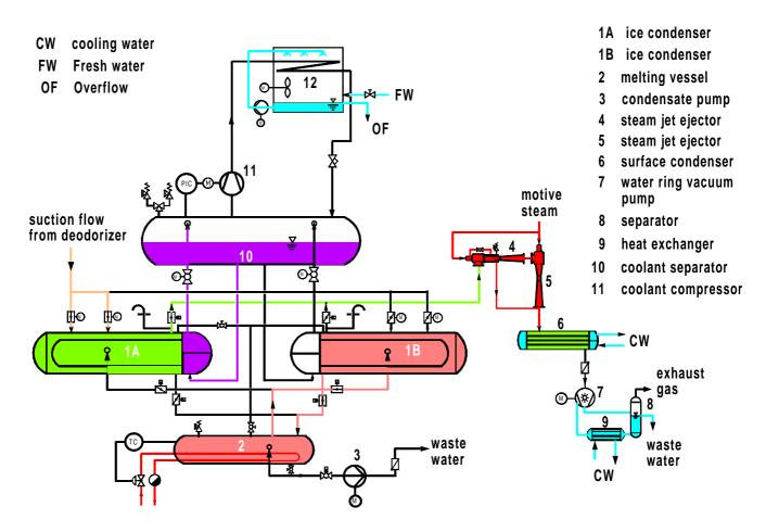
Following the idea to condense the stripping steam at the lowest possible temperature and pressure leads to a system where the stripping steam can be condensed at the process working pressure of the column. In case this pressure is below 6 mbar, water vapour condenses into the ice phase.
