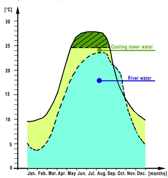
The possibility of condensing the water vapour (suction- and motive flow), depends on the temperature of the coolant, which is mainly cooling water.
