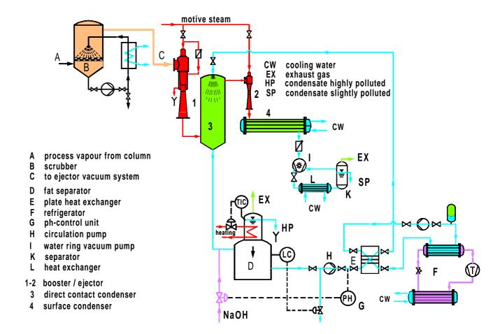
With the help of a refrigeration system the circulating water is cooled to about 4...6 °C and is warmed by about 3...4 °C in the mixing condenser
