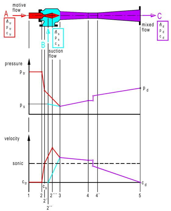
The motive flow enters the motive nozzle with a fixed pressure and velocity. It is not possible to transfer the high energy of the motive flow directly to the suction flow.
